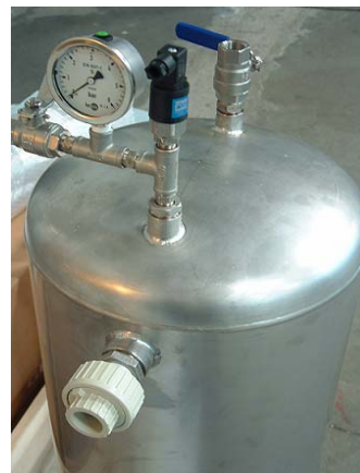
Photo: Ozonation tank.
